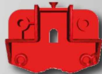
Short shots of electrical housing – Comparison Experiment vs Rem3D® simulation (in red)
