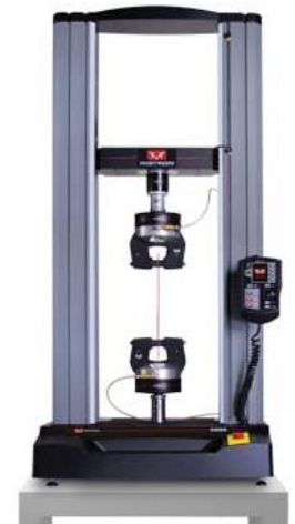
Instron 5966 Mechanical properties
