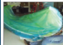
After the skin is laid up onto the FDM core, the composite is placed into a vacuum bag.
