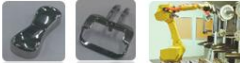
MIM Fine Powder High gross, High polishing, Mirror polishing by robot
