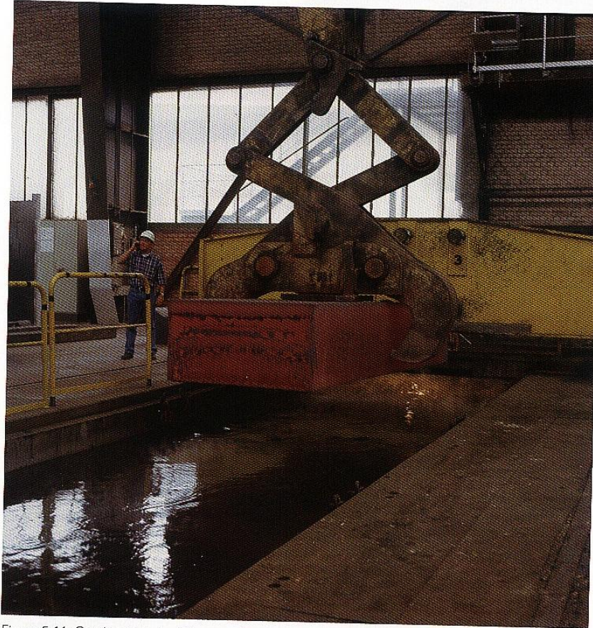
Figure 5.11: Steel ingot poised for quenching in the polymer pond at Edelstahlwerke Buderus AG
