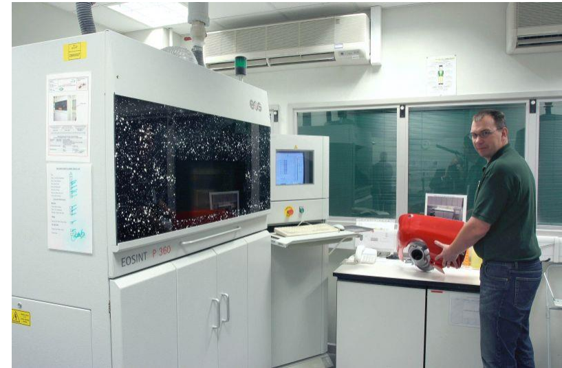
Laser-sintered prototyp produced in polyamid, painted afterwards, for assembly tests of key components e.g. exhaust pipes
