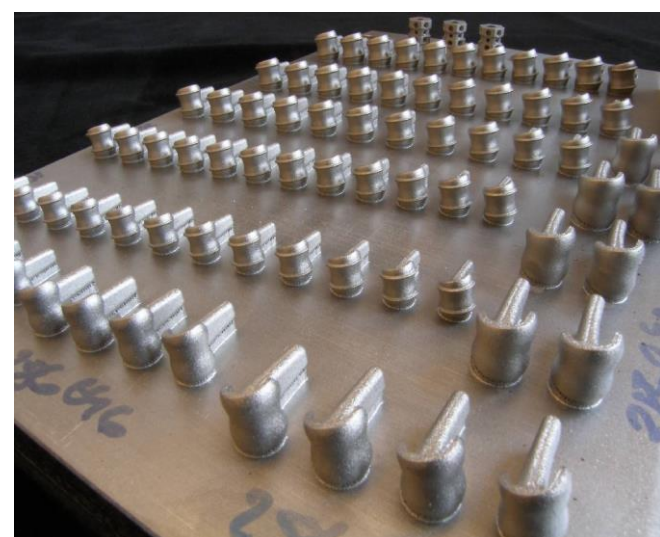
Batch of finger implants in EOS CobaltChrome MP1
