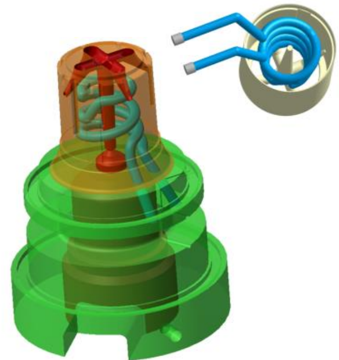
conformal cooling channel; design of the DMLS insert
