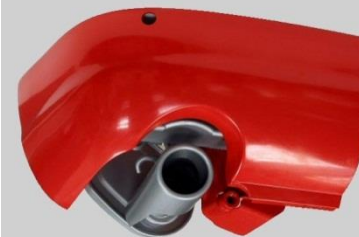
Laser-sintered prototyp produced in polyamid, painted afterwards, for assembly tests of key components e.g. exhaust pipes
