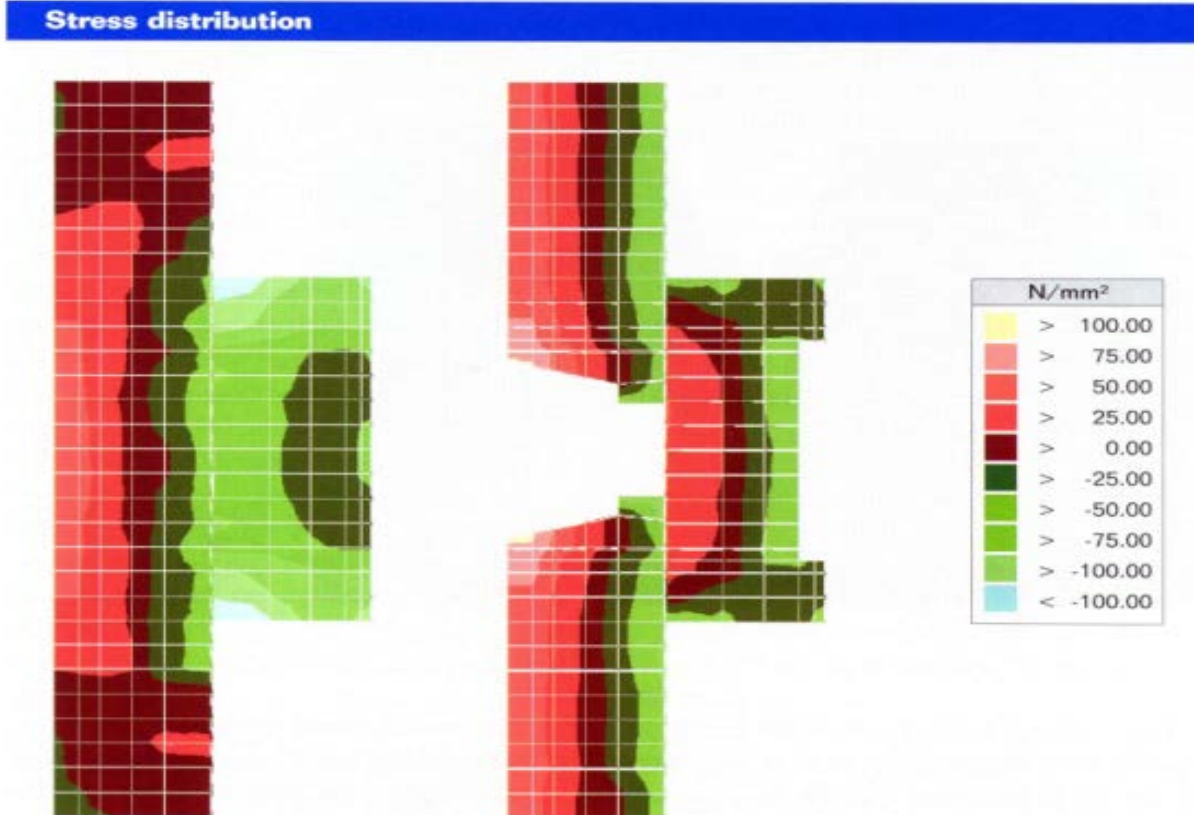
Figure 3.14: Stress distribution at the surface and in the cross section of the fixed clamping plate and the mould
